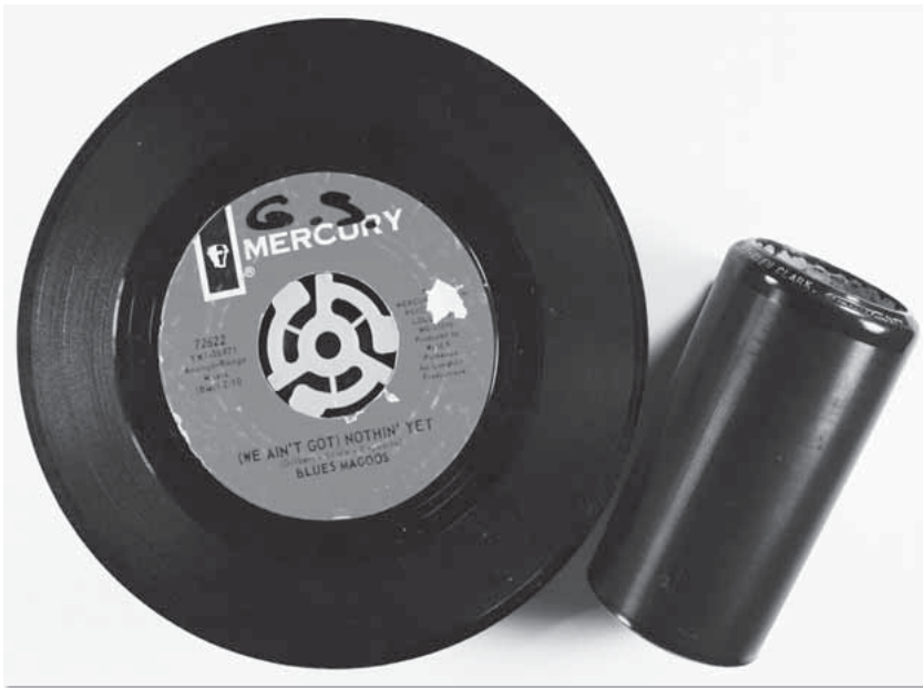
Polyvinyl chloride 45 rpm record and Edison Ambercol recording cylinder. Courtesy of Julianne Snider.
