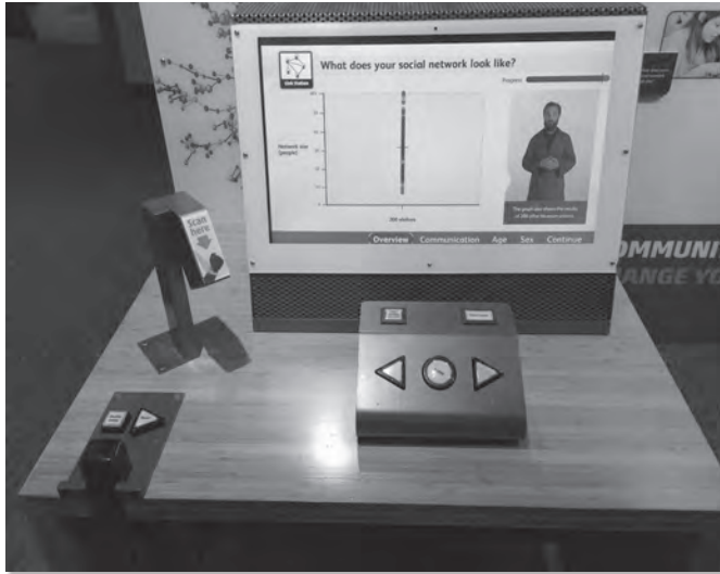
Fig. 3. Link Stations are controlled by “next,” “back,” and “select” buttons. After visitors answer a few simple questions about themselves, they find out where they stand in relation to previous museum visitors (via graphs and an on-screen guide). Photo by Sara Smith
