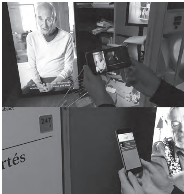
Fig. 6. The UAP (Universal Access Point) is a system of components that include a tactile floor marker, a tactile wall square, a low-energy Bluetooth beacon, and the museum’s mobile app. The UAPs provide access to static content that might otherwise be inaccessible to blind or sight-impaired visitors. Courtesy of the Canadian Museum for Human Rights
